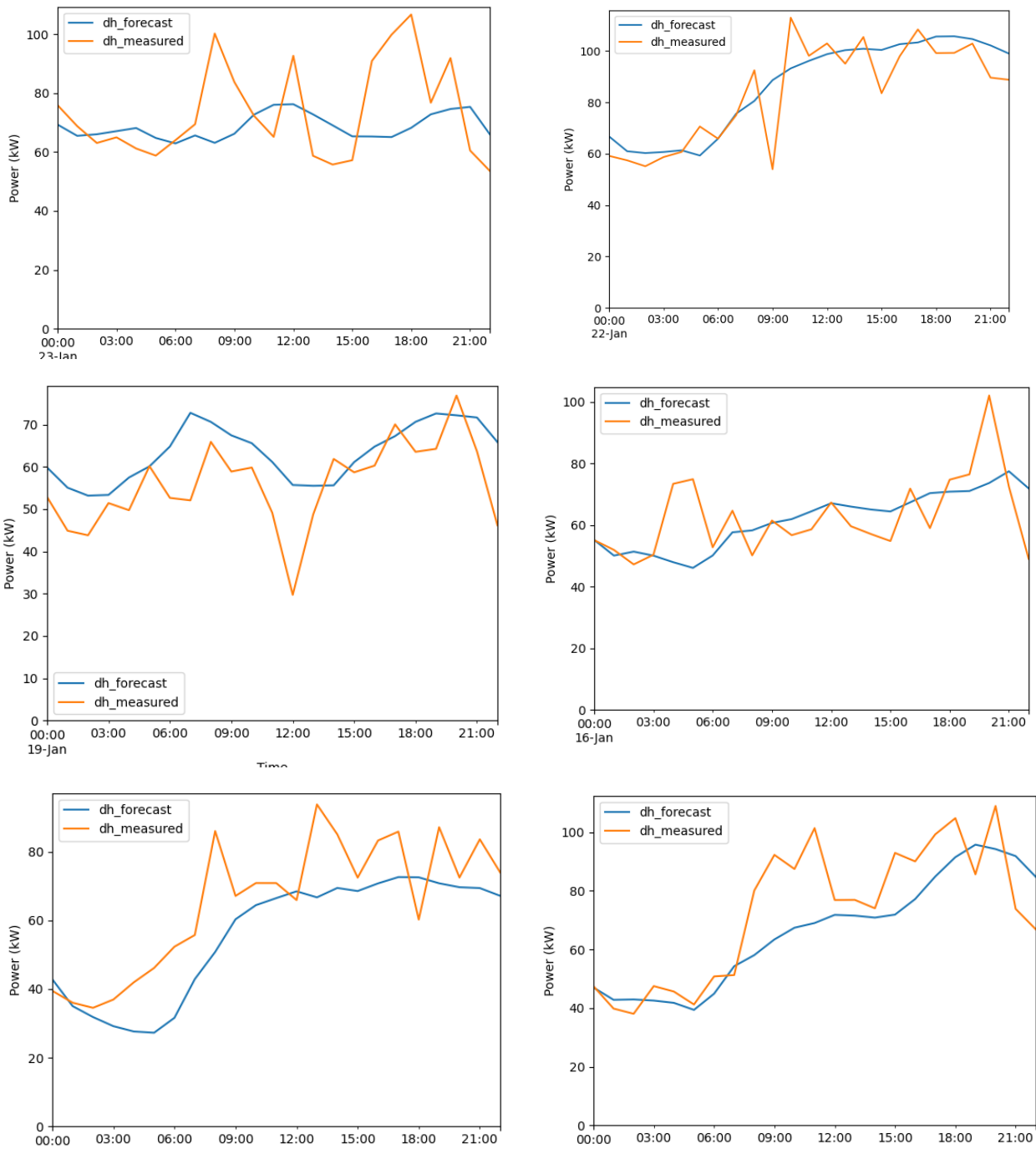
Figure 12: 24-hour district heating baseline load forecasts. Measured values are represented in orange and forecasts in blue.
